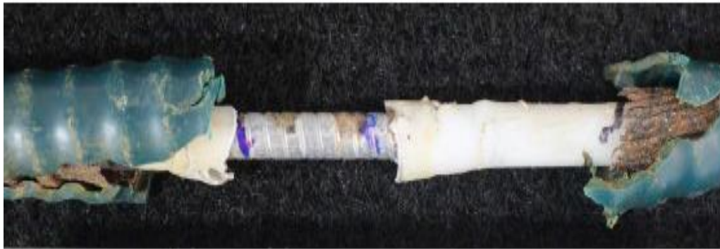
After a tragic lifeboat accident on the offshore production facility AUGER claimed two lives, the Coast Guard led a diverse investigative team to identify potential causal factors and prevent future casualties. Using independent laboratories, the team found that control cable sheathing damage could trigger inadvertent lifeboat deployments, which may have contributed to the casualty on the AUGER. (Coast Guard Photo)
