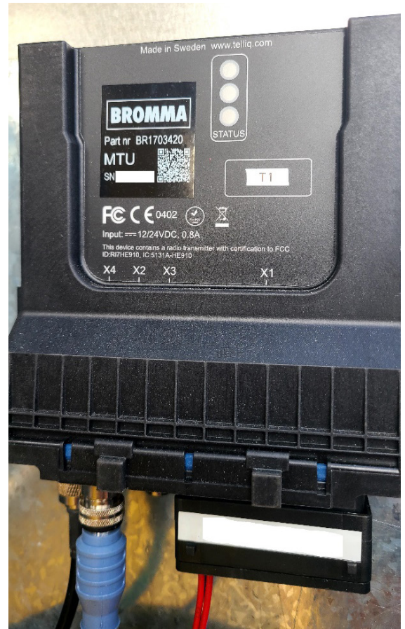
A cellular modem installed on a crane's spreader
