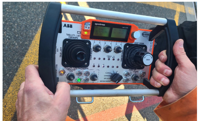
Image of an ABB manufactured crane remote controller for ZPMC STS cranes
