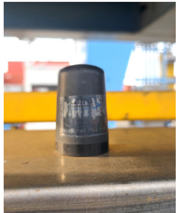
Cellular modem antenna installed on a crane's spreader system
