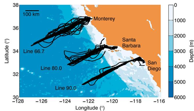
**Figure 1.** Glider profile locations from October 2006 to June 2015 along CalCOFI lines 66.7, 80, and 90 in black. Blue and tan contours show bathymetry and land, respectively.
