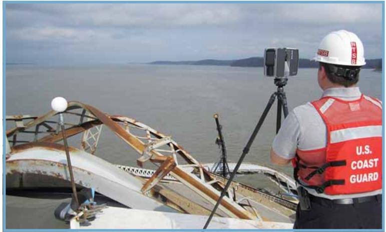
A technician from the NTSB uses a sophisticated laser imaging device to map the twisted steel on the bow of the M/V *Delta Mariner* while wearing a Coast Guard flotation device and an NTSB hard hat, suggesting the epitome of collaboration. Photo courtesy of the NTSB.
