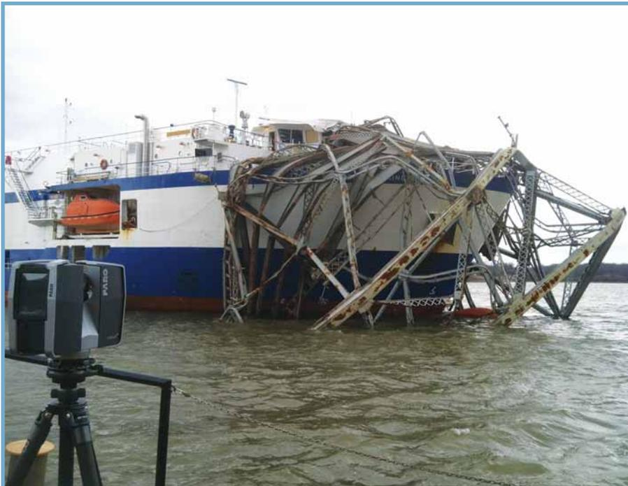
The bow of the *M/V Delta Mariner* with the twisted span of the Eggner's Ferry Bridge anchoring the ship to the bottom. The ship was specifically designed to be able to pass under bridges on the inland waterways. Photo courtesy of the NTSB.
